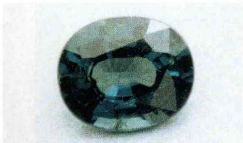
Figure 5: Almost blue garnet from Madagascar (sample J, group I) in daylight. This sample displays only a very slight change of colour hue when examined under tungsten light. Photo by M.S. Krzemnicki, © SSEF.
