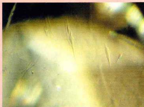
Figure 4: Oriented lozenge-shaped or needle-like crystals, some with a distinct jagged outline. Dark field, fibre optic illumination, magnified 100x. Photomicrograph by E. Gübelin.
