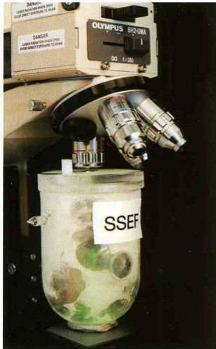
The Raman microscope at SSEF Swiss Gemmological Institute for taking supercooled luminescence spectra of diamonds.
