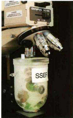
The Raman microscope at SSEF Swiss Gemmological Institute for taking supercooled luminescence spectra of diamonds.
