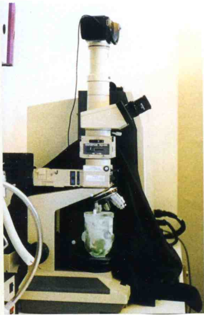
RENISHAW Raman Microscope System with cryogenic sample stage at SSEF
