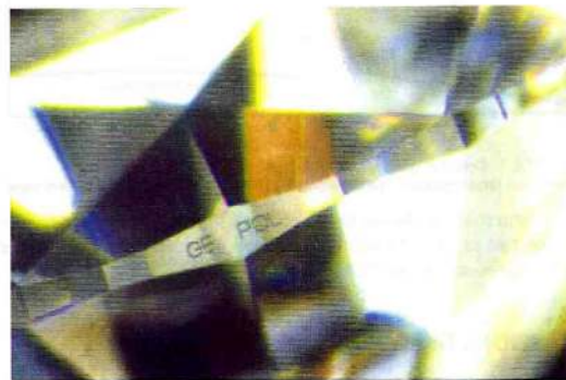
GE POL is laser inscribed on the girdle of HPHT treated diamond
