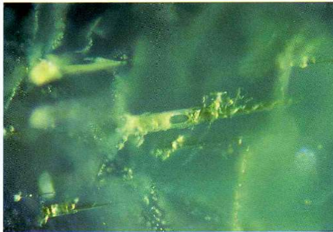
Figure 8: Elongated channel parallel to the c-axis with multicomponent filling and shrinking bubble. Renishaw Raman microscope. 200x.
