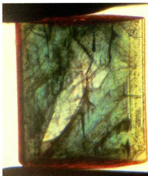
Figure 2: Prismatic crystal of Nacken synthetic emerald which contains a colourless, natural irregularly-shaped seed; the c -axis runs vertically, melt filled channels and spicules are oriented parallel to c . Immersion, length of crystal 2 mm.
