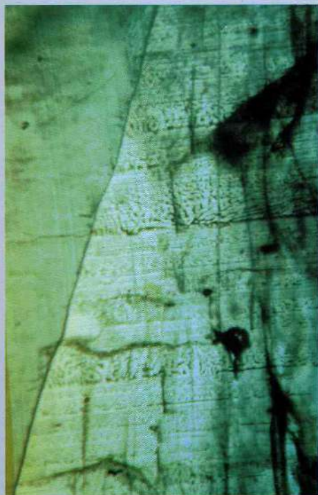
Figure 12: Growth pattern of Chatham synthetic emerald consisting of growth sectors related to the basal pinacoid (right) and to a prism face (left); nailhead spicules occur in the basal growth sector. The c -axis runs vertically, immersion, 50x.
