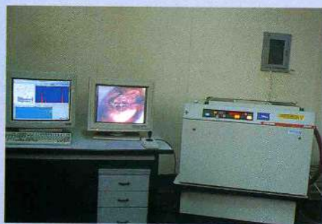
Figure 3: The OMICRON XRMF analysis system consisting of the basic measurement unit (right) colour TV sample display (centre) and computer-based data processor (left).
