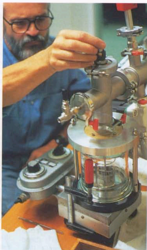
Figure 1: Vacuum chamber on heating stage. This system is in use at the Institute of Earth Sciences of Basel University for hardening porous rocks to make them workable. For emerald treatment, the cleaned stones are evacuated above the filler, and then lowered into the substance. Normal pressure is admitted when the liquid has penetrated into all open fissures and fractures. © SSEF Swiss Gemmological Institute.
