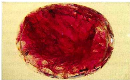
Figure 4. Natural corundum with an artificial red colouration. The deposition of red dye follows the irregular fracture planes. (2.5x)
