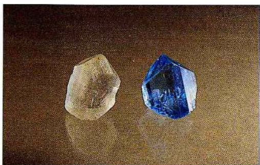
Figure 9. Two natural topaz crystals where the colourless one shows its original colour (left). The blue crystal has a treated colour (right) due to irradiation. Length of the crystals is approximately 2 cm.
