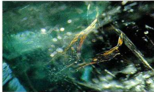
Figure 7. Orange and purplish flashes indicate the presence of artificial resin in this treated emerald. The identification of this observation needs instrumental confirmation e.g. by FTIR or Raman spectrometry. (60x)
