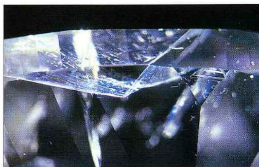
Figure 1. Cleavage planes and fissures in this brilliant-cut diamond show a slightly milky appearance together with multicoloured flashes. Tiny gas bubbles are also an indication of the artificial foreign substance used for enhancement. (40x)
