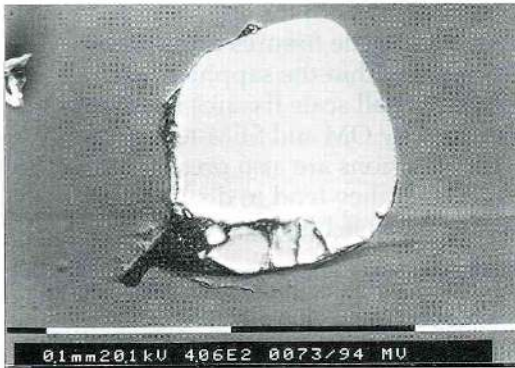
Fig. 15. BSE micrograph (SEM) of a syngenetic Fe-Zn-Al-spinel.
