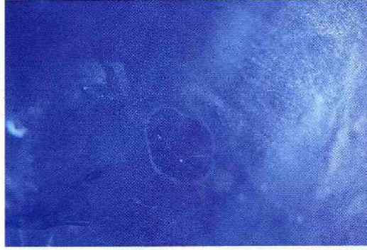
Fig. 17. Stress fissures (atoll-structure) around microscopic zircon inclusions.
