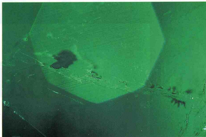
Picture four: extension of the fracture into the stone. Fracture filling becomes visible due to partial dark field illumination
