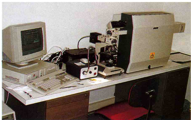
Picture one: a Renishaw Raman microscope with the laser source behind the spectrometer box. This system is operated at the SSEF Swiss Gemmological Institute in Basel, Switzerland
