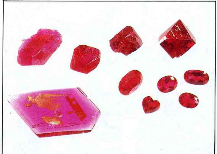
Picture two: most of the crystals possess a rhombohedral shape, upper right. A typical tabular crystal with coarse flux inclusion is on the lower left, and a cluster is shown in the upper left. Largest crystal is 3cm across
