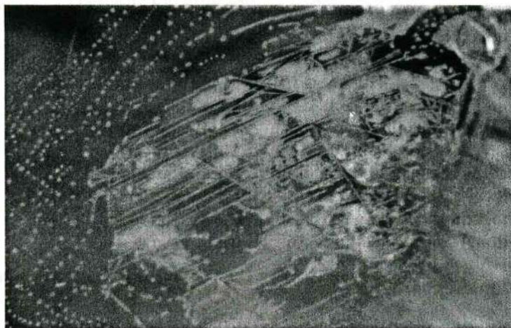
This artificially healed fracture has recrystallized under the flux effect of the glass. In newly formed crystalline cells, the glass has been trapped, devitrified, and formed white radiating crystals.
