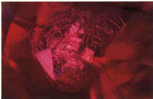
Fig. 7. Artificially healed fracture in a ruby. Under the flux effect of the glass the fracture plane has recrystallized. In newly formed crystalline cells, the glass has been trapped, devitrified and formed bunches of white radiating crystals. Magnification 40x.
