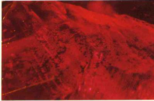
Fig. 4. Ruby with a fracture, probably treated with wax or paraffin. A typical dendrite-like pattern is visible.
