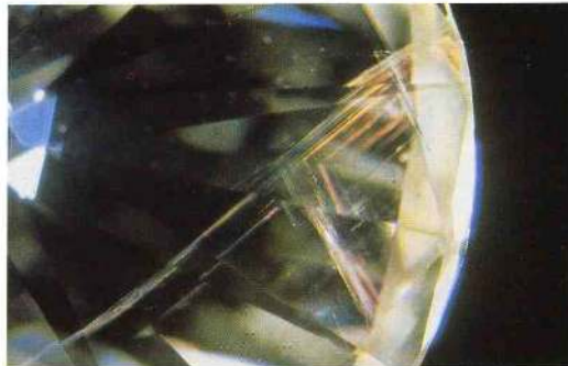
Fig. 8. Treated cleavage fractures in a brilliant-cut diamond. Yellow and violet interference colours together with gas bodies are characteristic for the Yehuda treatment.
