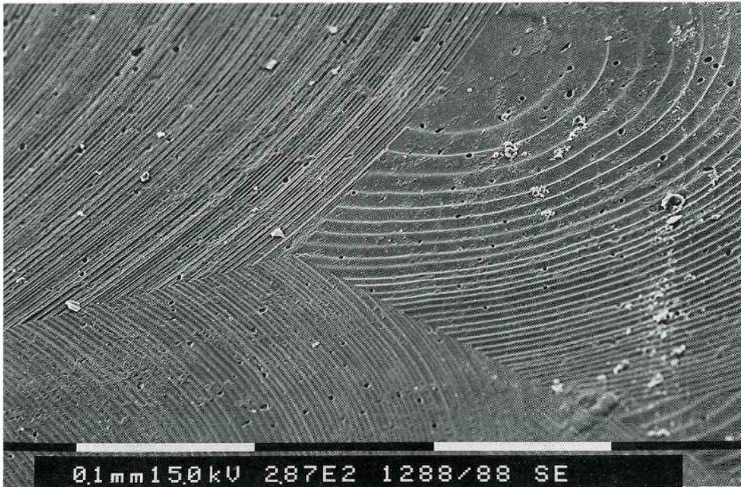
Fig. 6. SEM micrograph of the surface of a raw sample of iridescent glass revealing thin and bent layers as well as a few holes. White scale bar is 0.1mm long.
