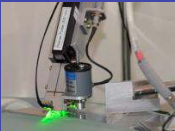
Laser source and Raman probe for sorting out of diamond imitations Electromagnetic arm for rejecting any diamond-imitations
