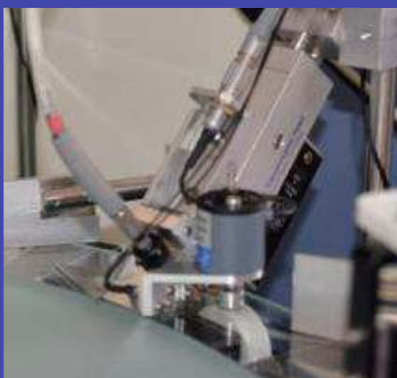
UVSW diode source and the optic fiber conducting the signal to a spectrometer for sorting out UVSW transparent diamonds.
