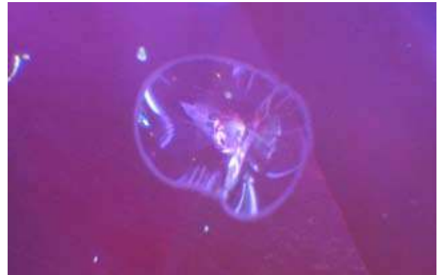
Fig. 2: Atoll-like structure of a molten inclusion due to heating. These features are only seen in pink sapphires heated at about 1000 °C. Below that temperature, clear microscopic evidence of heating is often missing. © M.S. Krzemnicki, SSEF
