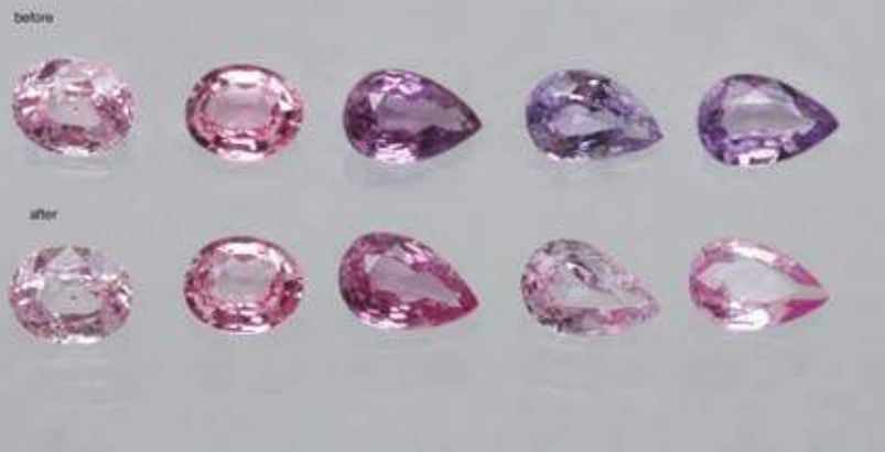
Fig. 1: A series of pink sapphires from Madagascar before (above) and after (below) heating at 1000 °C. The heating has had an obvious effect on the colour of these stones, removing the blue component and making them more attractive for the trade. © M.S. Krzemnicki,
