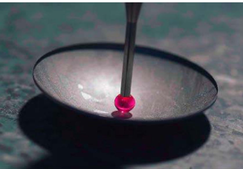
Fig. 2: This polycrystalline CVD synthetic diamond dome (26.29 mm across) is a high-tech component of the 800 series HiFi loudspeaker produced by Bowers & Wilkins. The picture shows the control measurement of the thickness. Photo source : Bowers & Wilkins
