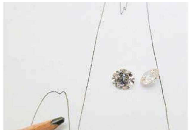
Fig. 3: Small brilliant cut CVD synthetic diamonds (approx. weight 0.70 ct each), analysed in detail at the Swiss Gemmological Institute. © SSEF
