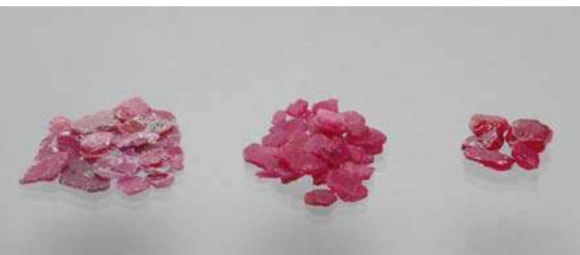
Fig. 5: Ruby crystals from Montepuez in Mozambique: Unheated, heated with borax and heated with Pb-glass. © M.S. Krzemnicki, SSEF.
