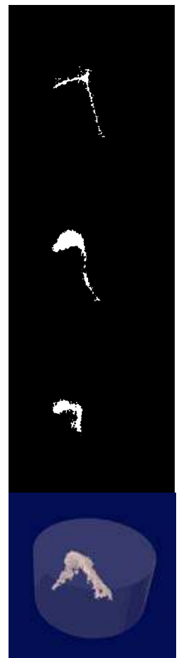
Fig. 4: Three different cross sections through the beadless cultured pearl (see above). The white structure shows the curved „moustache“ structure of this pearl. The figure at the bottom show a a three dimensional model of the characteristic structure for this beadless cultured pearl. . © M.S. Krzemnicki & P. Chalus, SSEF and Roche (Basel).
