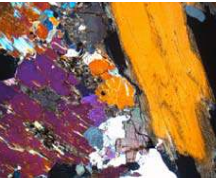
Fig. 4: Thin section of the parent rock of the Montepuez deposit under crossed polarizers: amphibol (multicoloured grains), kyanite (orange-yellow) and Fe-carbonate (pastel colours with distinct cleavage) in polarised light. Width of image approx. 6 mm. Photo © Leander Franz, Mineral.-Petrogr. Institute, University Basel.
