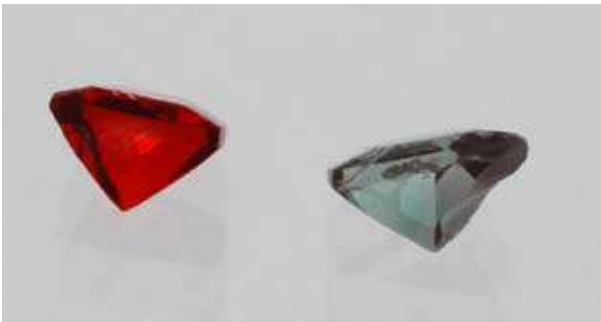
Red and green labradorite analysed with LA-ICP-MS to gain insight in the copper concentration of these feldspars. © M.S. Krzemnicki, SSEF 2008
