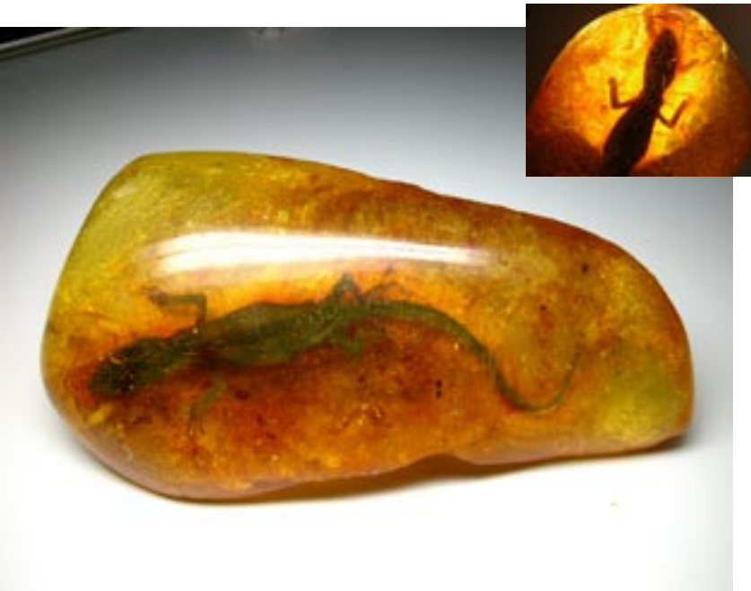
Fig. 1: This most unusual sample (15 x 8 x 2.5 cm) proved to consist of a modern lizard that was artificially embedded in a natural resin.
