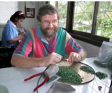
Fig.5 Werner Spaltenstein trimming with tongs rough tsavorite (vanadium grossular garnet) in Chanthaburi. © H.A. Hänni, SSEF 2005
