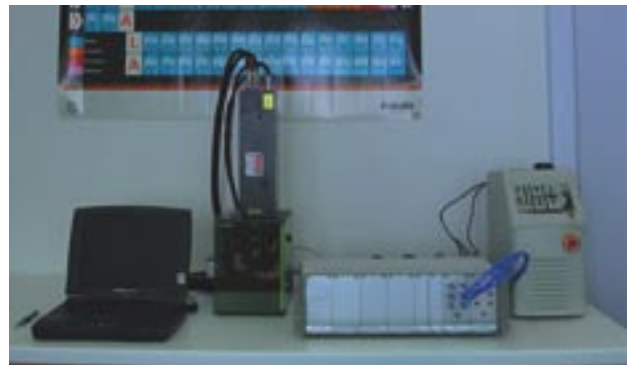
The SSEF GemLIBS system in the laboratory of the Swiss Gemmological Institute SSEF. The system consists of a sample chamber with attached laser (centre), the high resolution fibre optic spectrometers, the laser power supply (right), and a computer for system control (left). © H.A. Hänni, SSEF 2004
