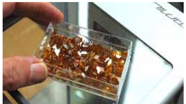
Orange yellow HPHT synthetic diamonds from the Ziemer factory in Nidau, Switzerland.
