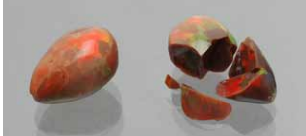
Figure 1: Two of the investigated stabilized opals from Shewa, one broken (right), one still in shape (left).
