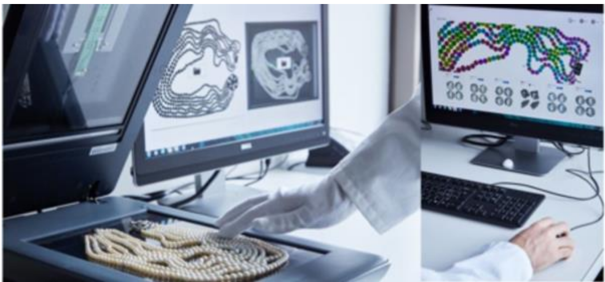
PearlScan® system (left) and user interface (right) for documenting and measuring single and multi-strand pearl necklaces. Photo: SSEF
