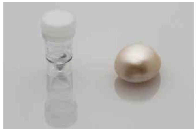
△ Figure 2: Plastic tube containing a minute amount of nacre powder together with the cultured saltwater pearl from which it was extracted (sampling along the drill-hole at the backside of the pearl). Radiocarbon age dating revealed this cultured pearl ( Pinctada maxima ) to be of rather recent age with a 90% probability to have formed between 1993 and 1996. Photo: SSEF
