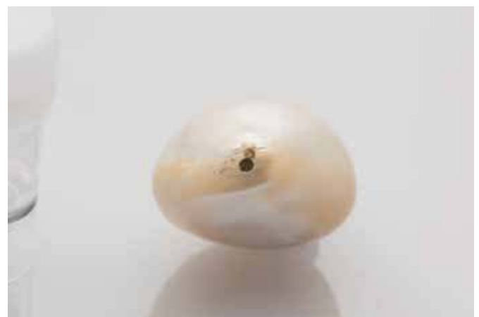
△ Figure 3: As the existing drill hole in this pearl was blocked with a metal lining (glued into drill-hole), we had to drill a small shallow additional drill-hole (diameter 1mm) to extract enough nacre for age dating of this pearl. Photo: SSEF
