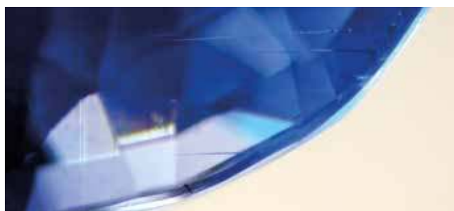
△ Figure 4: Fine corroded hollow channels at the girdle of this sapphire from Ambatondrazaka. Photo: M.S. Krzemnicki, SSEF
