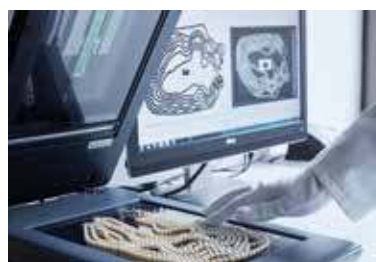
◁ Figure 1: The PearlScan® system: a scanner to acquire pearl image data, a computer to perform the assessment and measurement, and a user interface to present results and allow user input. Photo: SSEF
