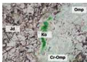
△ Thin section photo of a foliated shear band containing kosmochlor aggregates (vivid green), slightly greenish Cr-omphacite, and omphacite, which cuts through the coarse-grained jadeite matrix. Photo: © K. Ernst, University of Basel
