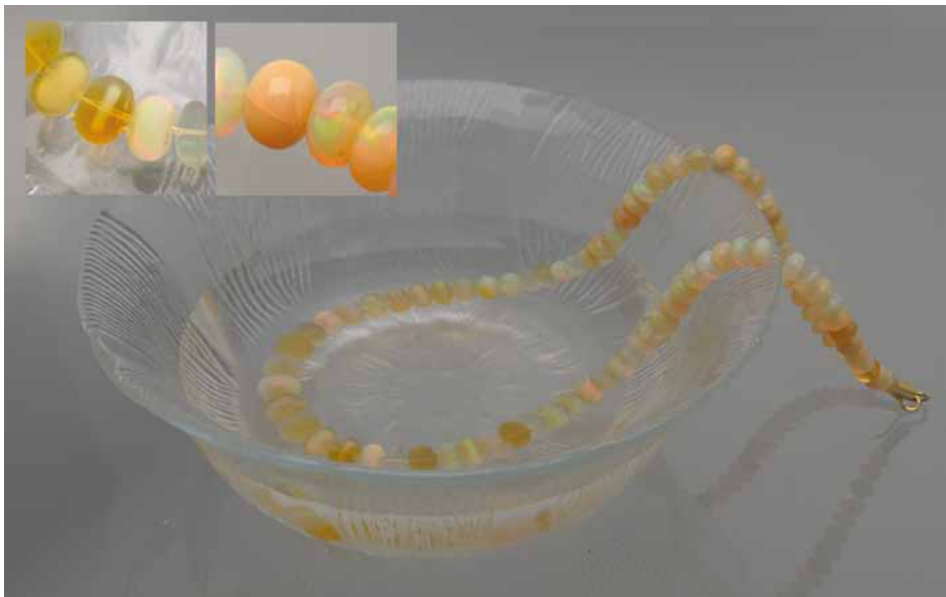
△ Opal necklace partially immersed in water for a stability test. Small inset photo on the left shows the situation after three hours in immersion, with a whitish core surrounded by a transparent rim. Small inset photo on the right shows a newly developed crack in an opal bead after drying. © M.S. Krzemnicki, SSEF
