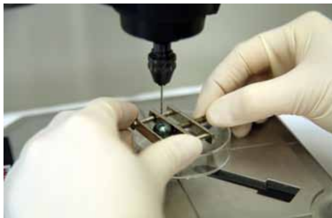
△ Figure 2: Pearls are drilled in a practically non-destructive manner to extract material that contains oyster DNA
