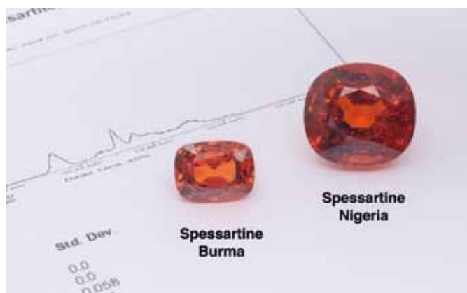
△ Spessartine garnet from Burma and Nigeria (34 ct), arranged on the print out of the chemical analysis (EDXRF) of the Nigerian sample. The main peaks in the XRF-spectrum are due to the presence of manganese within their crystal structure. Photo © M.S. Krzemnicki, SSEF
