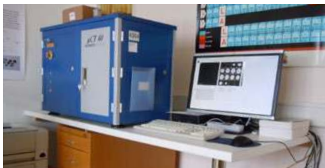
△ Our Scanco µCT 40 Scanner at work: The blue "box" is the actual scanner with some sample holders on top, and right to it is the screen of the computer. This computer is a HP workstation running the reliable VMS-operating system, that allows for very comfortable batch job handling.
