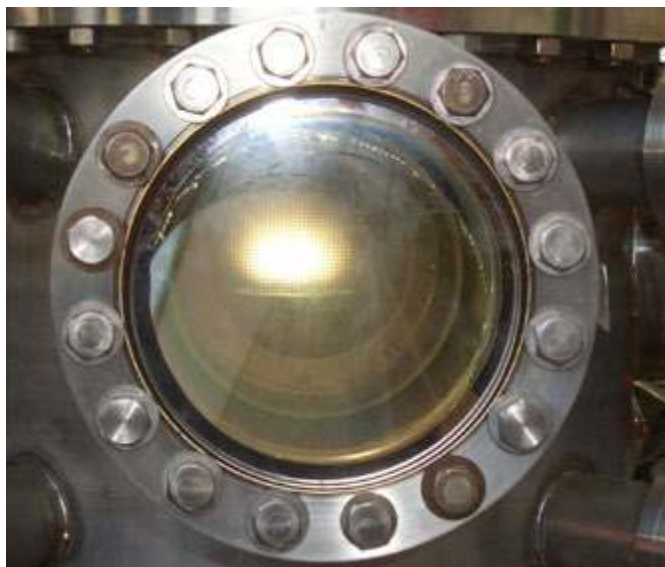
△ Plasma in which a CVD synthetic diamond is growing inside a microwave reactor at CNRS laboratories (LIMHP). Photo: SSEF.
