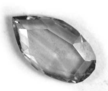
One of the CVD synthetic diamonds from Apollo Diamonds Company, USA, tested at SSEF Swiss Gemmological Institute
